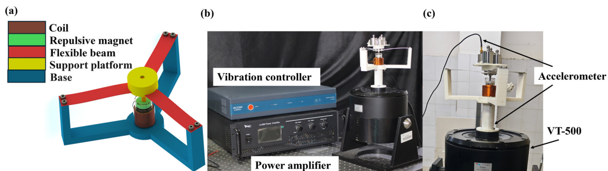
FIG. 1. The electromagnetic energy harvester system: (a) schematic diagram, (b) and (c) experimental setup.
