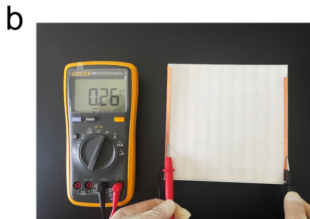
Figure S14: Measurement of the capacitance of the M-TENG (a) and the MO-TENG (b).
