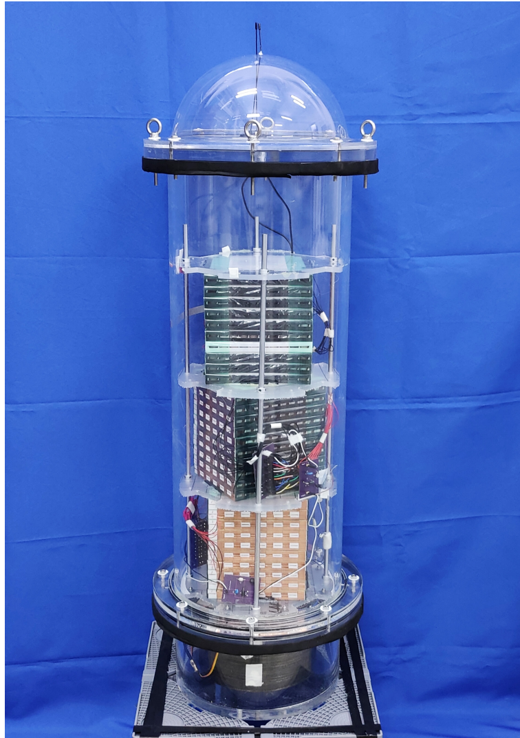
Figure S35: Photograph of the buoy stacked with 30 MO-TENG units.
